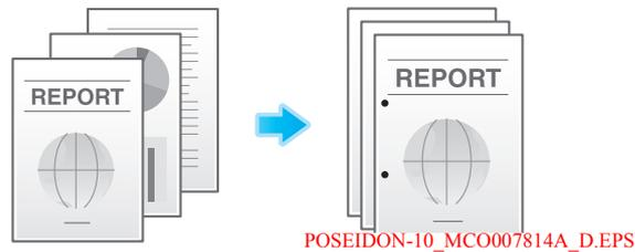
In the [Finish] tab, select the [Punch] check box. In addition, specify the number and positions of punch holes.
