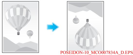
In [Layout / Finish], select the [Rotate 180] check box.
