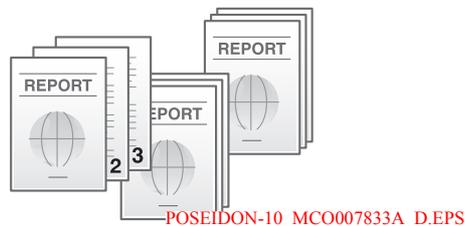
When the [Collate] check box on the [Basic] tab is selected, copies are output separately in a set-by-set manner, for example, "Pages 1, 2, 3, 4, and 5", "Pages 1, 2, 3, 4, and 5", and then "Pages 1, 2, 3, 4, and 5". When the [Offset] check box is selected, the sets are output in staggered layers.
