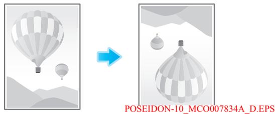
In the [Layout] tab, select the [Rotate 180] check box.
