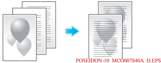
In [Overlay] in the [Stamp/Composition] tab, select [Print Host Image] or [Print Device Image] (PCL only), and then from the list, select the overlay image to be printed on the original as a composite image.
