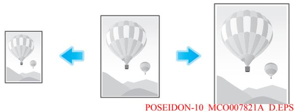
In [Paper Size] in the [Basic] tab, select the size of paper for printing. The zoom ratio is automatically determined by the paper sizes selected in [Original Size] and [Paper Size].
