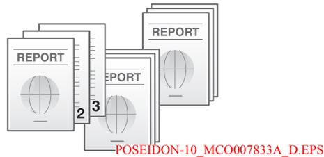
When the [Collate] check box in [Output Method] is selected, copies are output in a set-by-set manner, for example, "Pages 1, 2, 3, 4, and 5", "Pages 1, 2, 3, 4, and 5", and then "Pages 1, 2, 3, 4, and 5". When the [Offset] check box is selected, the sets are output in staggered layers.
